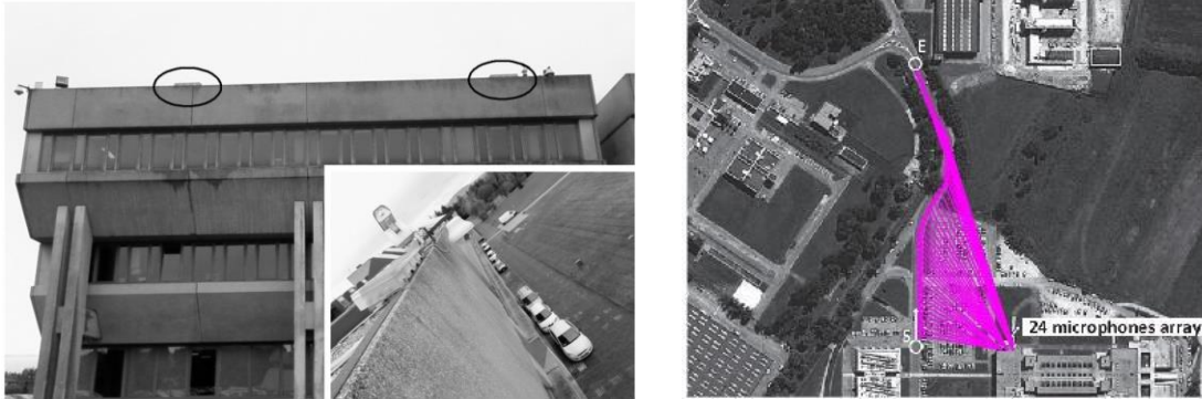
Figure 3: An example of microphone array configuration for outdoor acoustic source localization and tracking. Left: the sensor array configuration; Right: the acoustic tracking of a vehicle crossing the area under surveillance.
